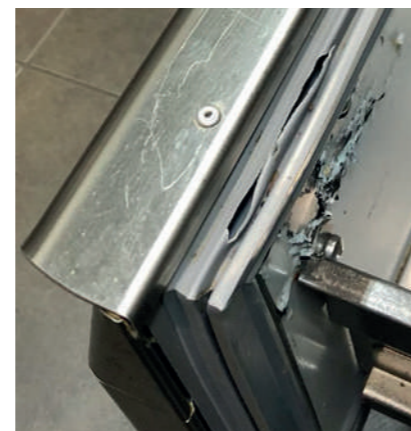
worn door seal
